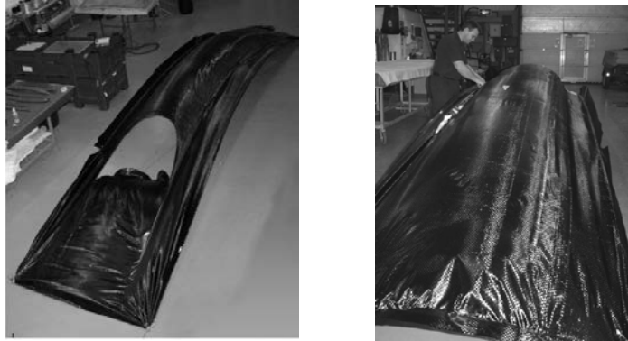
Fig.4: Large prototype incorporating various features. Pre-preg Carbon 0/90 Satin, 200 gr/m 2 . 3 plies+corner reinforcement
