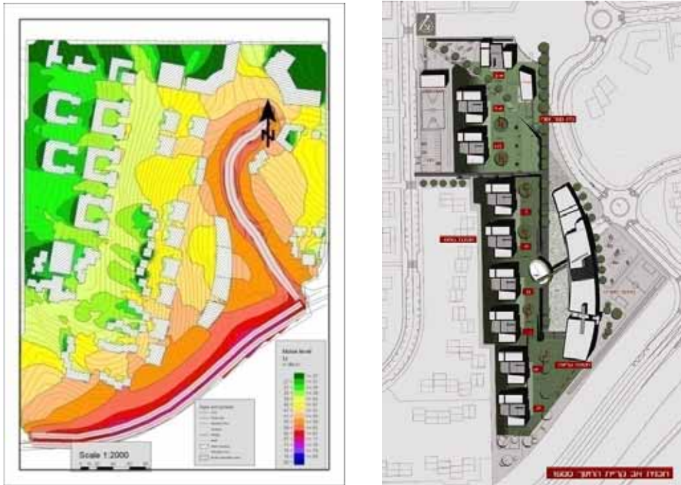
Figure 28 – Urban noise analysis using SoundPlan ( http://www.soundplan.com/ ). On the left, Acoustic simulation done by M.G. Acoustic for an entry to the Yokneam High school competition. On the right, entry to the Yokneam High school competition by Grobman Architects in collaboration with Lapidot Architects
