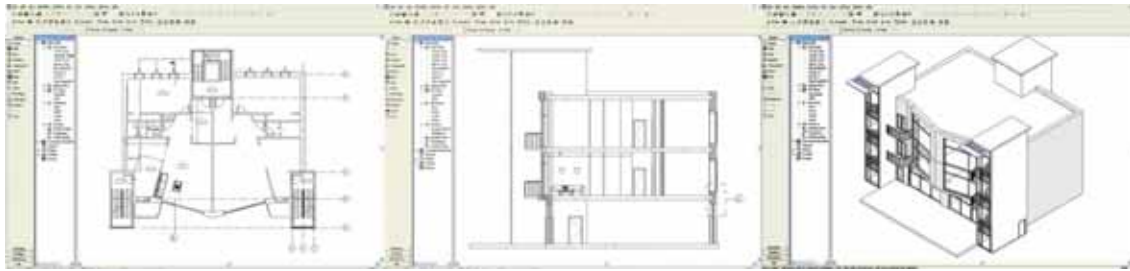
Figure 5 – Revit interface – One 3-D model is used to create plan and section documentation
